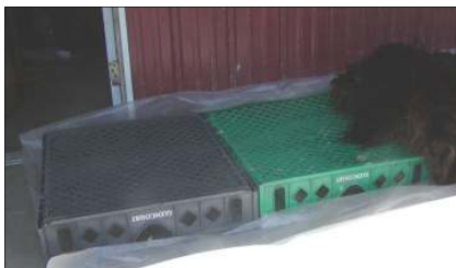
Racks are laid out at an angle over plastic (to catch moisture and excess salt).
